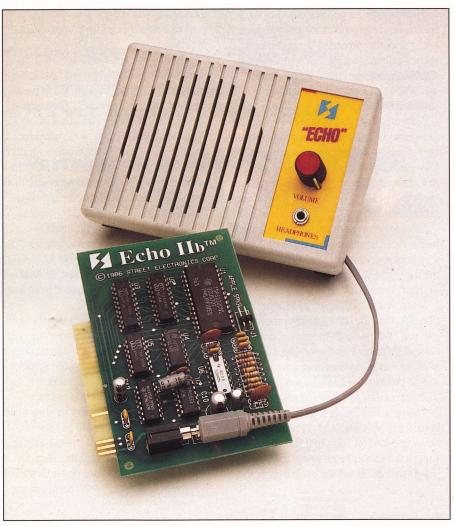
Play it again, ma'm. Using a proprietary speech chip, the Echo IIb board can enhance computer usage for preschoolers as well as the handicapped.
