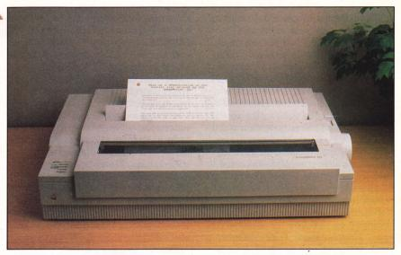
Driven by a 27-wire printbead, the ImageWriter LQ is more closely compatible with earlier software than 24-wire printers.
